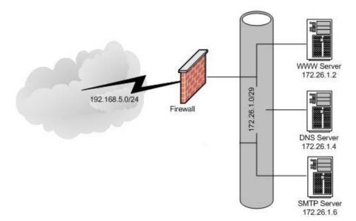
Here we have a typical DMZ with a firewall filtering inbound traffic. In our scenarios we will use "pseudo-rulesets" to keep the rules readable. The actual syntax from the rules are a mix between PF and engrish, so don't get hung up on the accuracy of them – they just need to be readable. Also, the version of nmap I used for this testing was 3.00
